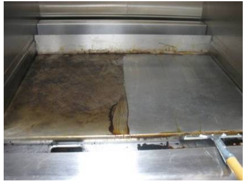
Squeegee product soils into the grease tray
