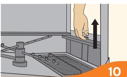
Lift drain lever and drain machine completely.
