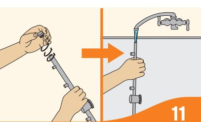
Unscrew top and bottom wash arms. Remove caps, then flush with water. Clean nozzles with toothpick and reassemble. Reinstall wash arms and ensure they spin freely.
