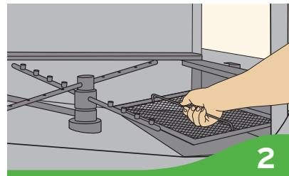
Check machine is clean and screens are in place.
