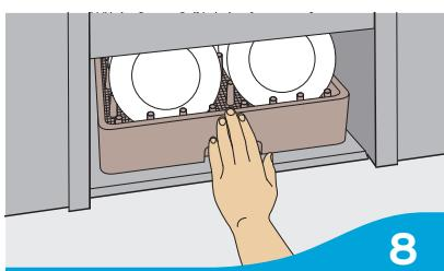
Load rack into machine and shut door. Do not remove rack until green "Cycle" light turns off.
