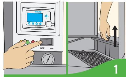
Check that machine is powered off and drained.
